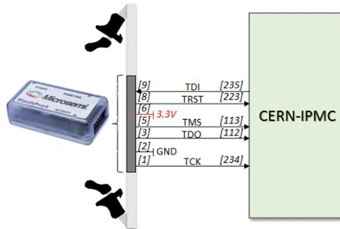
Figure 7: JTAG slave interface connectivity
