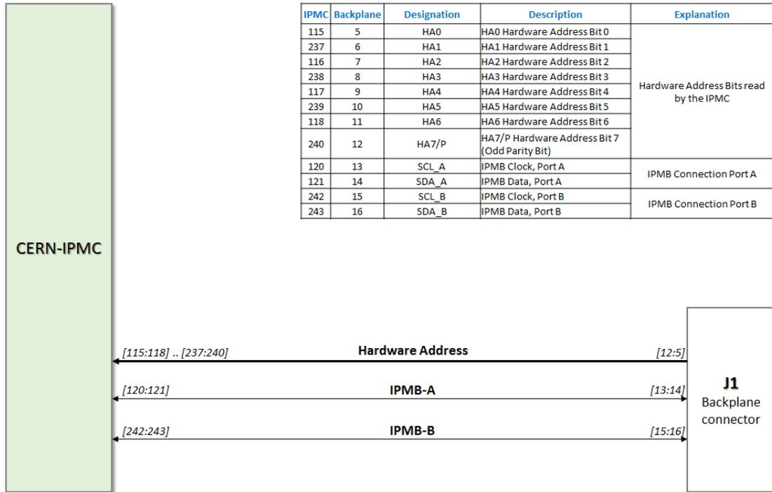
Figure 4: Zone1 interfaces connectivity
