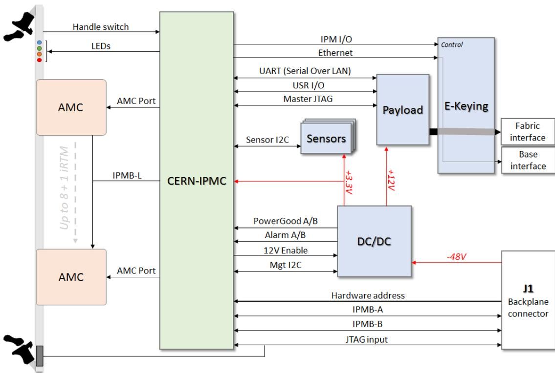
Figure 1: Typical use of the CERN-IPMC
