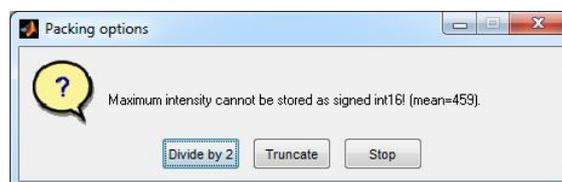
Typically high counts belong to the central transmitted beam or originate from hot spots and these intensities are not important. In this case the counts higher than 32,767 can be neglected (set to 32,767) using the truncate option. If the user decides to keep the intensity ratio also for the strong counts – all number can be divided by 2 in order to fit into the 0-32,767 range.
