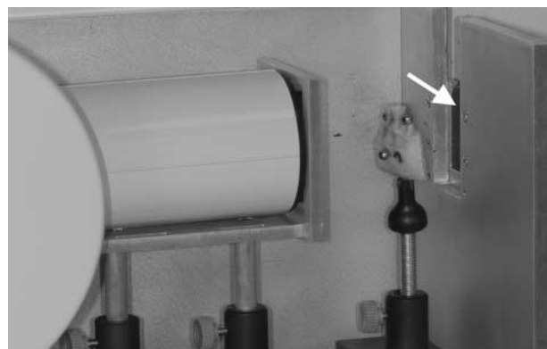
Figure 4 Experimental set-up on an optical bench, showing the specimen with the reference spheres attached in arbitrary, but non-collinear positions. Arrow indicates the position of the charge-coupled device (CCD)-sensor
