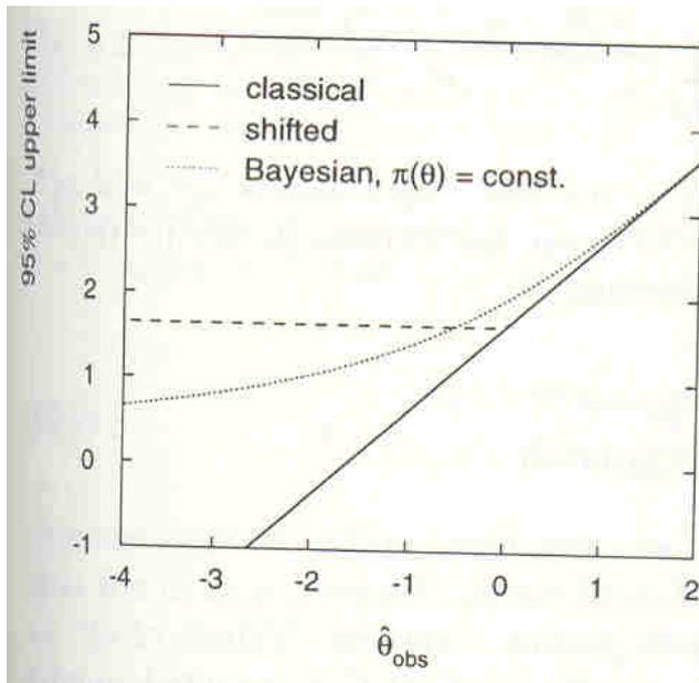
**Fig. 9.8** Upper limits at 95% confidence level for the example of Section 9.8 using the classical, shifted and Bayesian techniques. The shifted and classical techniques are equal for  $\hat{\theta}_{\text{obs}} \geq 0$ .
