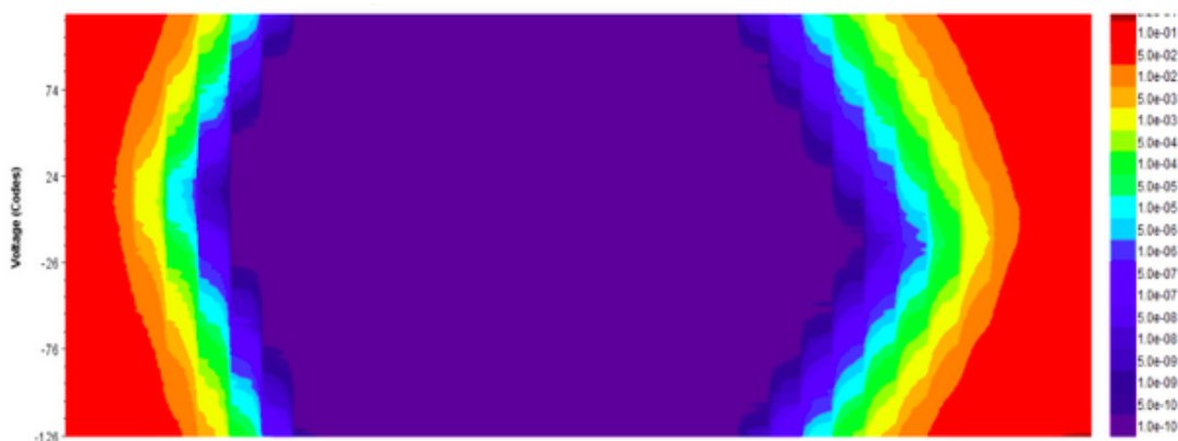
Figure 5.5: Finisar BOA IBERT loopback test: a typical eye diagram
