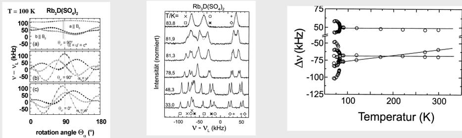
Resonance positions obtained by rotating about 3 mutually perpendicular axes for  $T > T_N$
