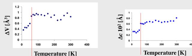
The difference between the lattice parameters of  $Rb_3D(SO_4)_2$  and  $Rb_3H(SO_4)_2$  exhibits a phase transition at  $\approx 80$  K.
