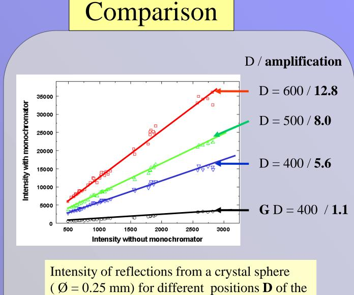
optic and for a graphite monochromator G versus the intensity without a monochromator
