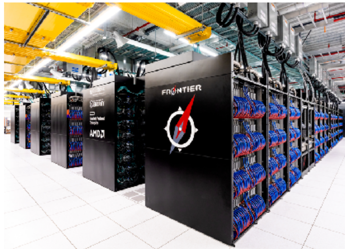
Frontier - HPE Cray EX235a, AMD Optimized 3rd Generation EPYC 64C 2GHz, AMD
