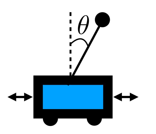
An unstable pendulum can be equilibrated with a moving cart which is controlled with an electric current.
