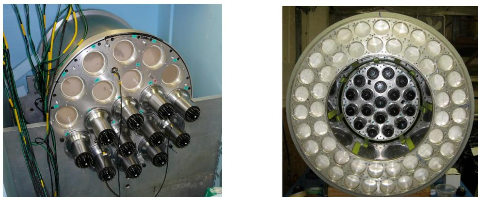
Figure 3.11: **(Left)** Back side of the NaI(Tl) crystal on the test bench. **(Right)** The NaI(Tl) crystal and the 97 pure CsI crystals while the calorimeter assembly was under construction in a low-humidity clean room at TRIUMF.
