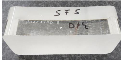
Figure F.1: SF5 Pb-Glass crystal (from Schott AG).
