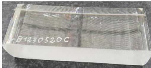
Figure F.2: SF6 Pb-Glass crystal (from Schott AG).
