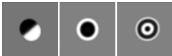
Fig. 58 Mean-field density profiles obtained from self-consistent field theory simulations. A- versus B-rich domains are displayed for a blend of A- and B-homopolymers ( a ) and for AB-diblock-copolymer melts ( b , c ). In each case, all A-, and B-blocks contain equal numbers of monomers. Here, spherical confinement is implemented by blending either A- and B-homopolymers ( a ), or AB-diblock-copolymers ( b , c ) with C-homopolymers. The C-homopolymers act as a very bad solvent, thus enforcing the formation of A-, and B-rich spherical domains. In this case, the geometry of the confined polymer phases is studied in two dimensions. Whether Janus ( a ), core-shell ( b ), or onion ( c ) particles form depends on the number of monomers per block, and the interactions between different monomer species. From ( a ) to ( c ), the length of A-, and B-sequences steadily decreases; the sequences in ( a ) are roughly four times as long as in ( b ), and are about 15 times as long as in ( c ). To form Janus particles, the A–C versus B–C interactions need to be equal. To form layered structures, there has to be a significant difference
