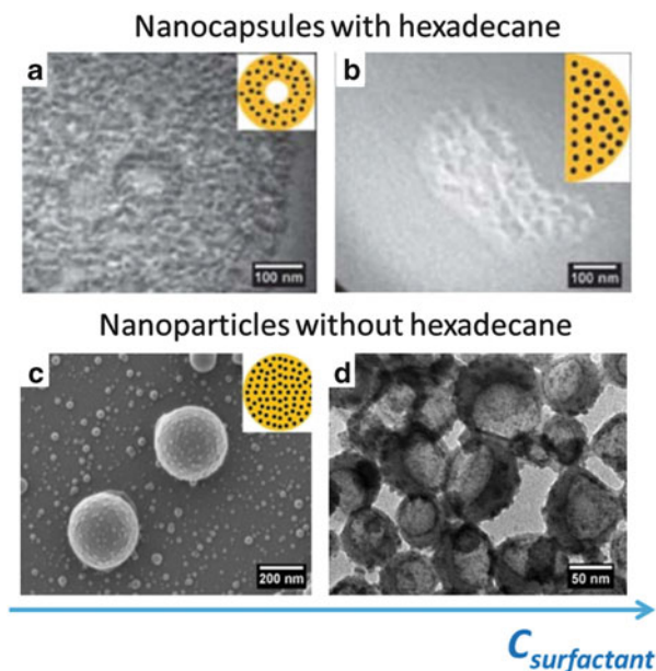
Fig. 57 Nanocapsules of PS_{76}\text{-}b\text{-}PMMA_{79} (weak segregation limit) show a structured surface in SEM and TEM images. In both cases, the small patches consist of PS, since it appears bright in the SEM and dark in the TEM. The patchy structure is also visible in TEM micrographs of stained cross-sections of (a) nanocapsules and (b) half-spherical nanoparticles and in (c) SEM and (d) TEM micrographs of nanoparticles consisting of PS_{76}\text{-}b\text{-}PMMA_{79} , indicating that it is not only a surface phenomenon [221]. Reproduced by permission of The Royal Society of Chemistry
