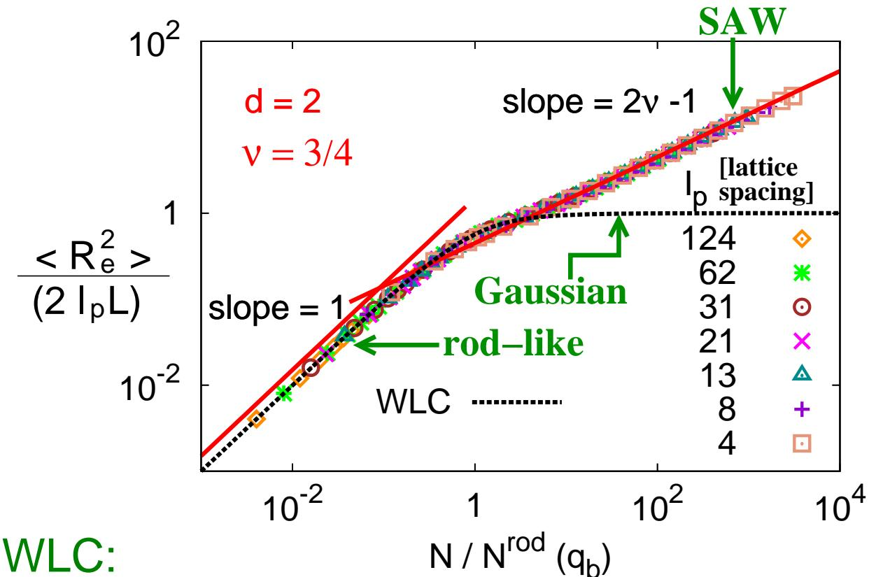
$$\frac{\langle R_e^2 \rangle}{2\ell_p L} = \begin{cases} L/2\ell_p = (\ell_b N)/(2\ell_p) & \text{for } L \ll \ell_p \text{ (rod-like chain)} \\ 1 & \text{for } L \rightarrow \infty \text{ (Gaussian chain)} \end{cases}$$
