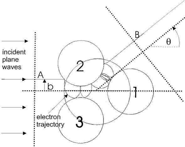
Fig. 1. Scattering geometry for the open three-disk billiard. The classical action  $S_j$  is calculated between the points A and B. The disks (radius  $r_d$ ) are arranged such that their centers form an equilateral triangle (side length  $a/r_d = 2.5$ ). The magnetic field  $B = \hbar k/qR$  (where  $R$  is the cyclotron radius) is assumed to be confined by a circle with radius  $r_B$ , which touches the corners of the triangle
