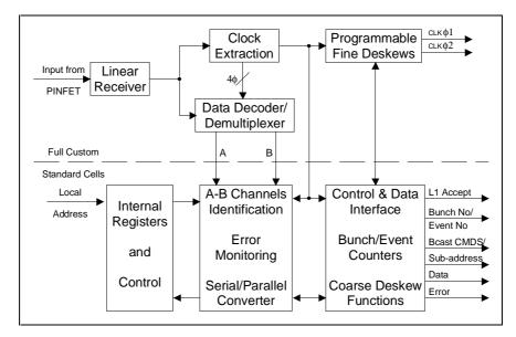
Figure 4 Timing receiver block diagram
