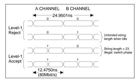
Figure 3 TDM biphase mark encoding
