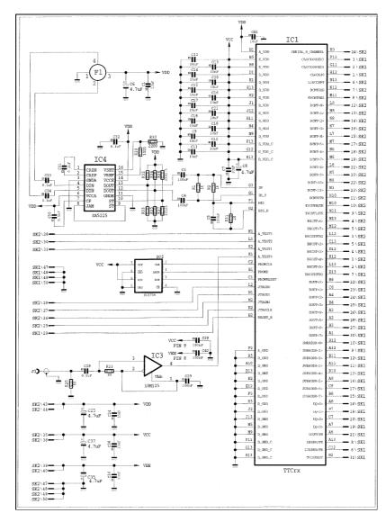
Figure 8 TTCrx test board schematic
