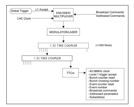
Figure 1 TTC optical distribution network
