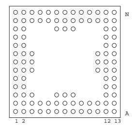
Figure 7 PGA100 package pin positions (bottom view)
