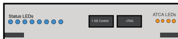
Figure 4. Preliminary front panel layout (not to scale).
