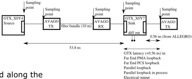
Latency measured along the real-time path in various points at 6.4 Gbs, 16 bit data width, and 8b/10b encoding
