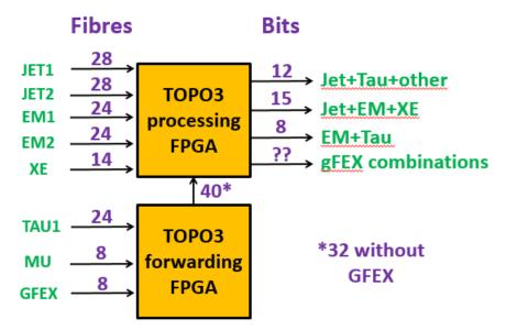
The general layout is similar, and there is still a need for inter-FPGA communication, but with fewer links even without preprocessing (32 links if gFEX combinations are not required). The output routing is still likely to require the fast electrical cable.
