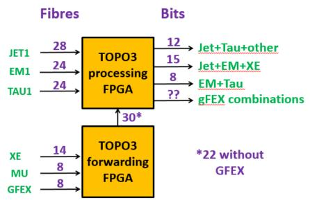
So an alternative scheme for TOPO3 can be devised as below.
