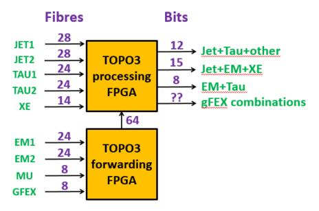
This illustrates that to implement some of the most complex algorithms, while also requiring all inputs from systems such as eFEX and jFEX, results in a very demanding input count into one FPGA. Other arrangements are possible which may spread this load, in particular by redistributing the algorithms between TOPO2 and TOPO3. However, an algorithm that requires all EM, Tau and Jet TOBs will inevitably need to have 152 inputs, and will be difficult to accommodate in any layout.
