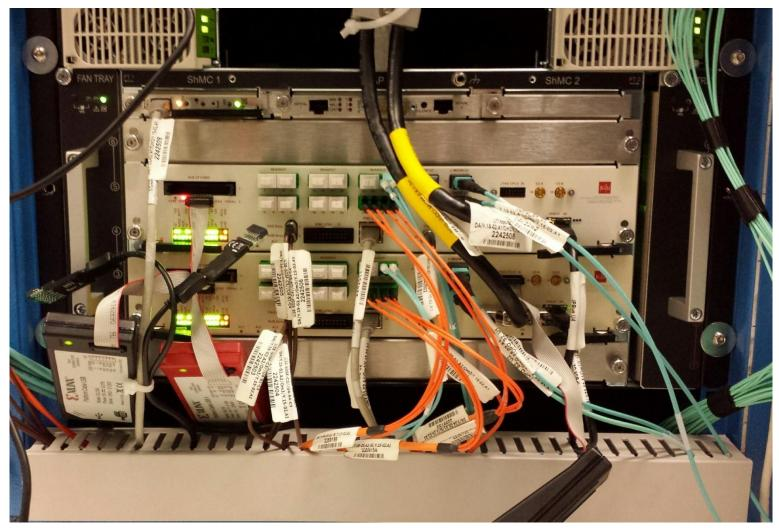
Two modules running topological algorithms, Calo & Muons (multiplicity based Calo triggers provided by CMX)
