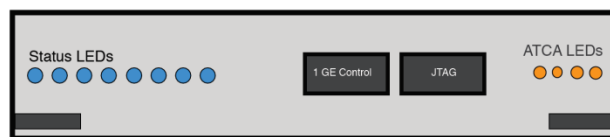
Figure 4. Preliminary front panel layout (not to scale).
