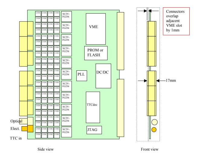
Current consumption at 3.3V. 88 LVDS serialisers @40MHz, Total = 4.2 A. FPGA consumption?
